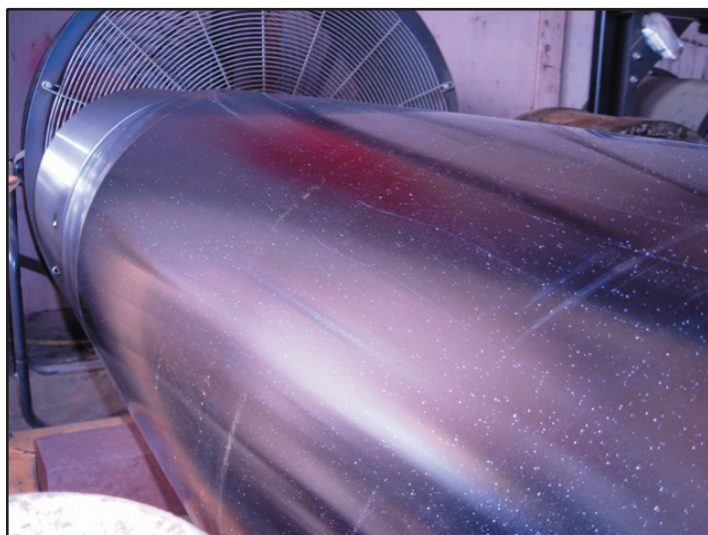
Exhibit 5-11. Long shaft with thousands of pits after plating. These pits were caused by inadequate pre-plate grinding.
