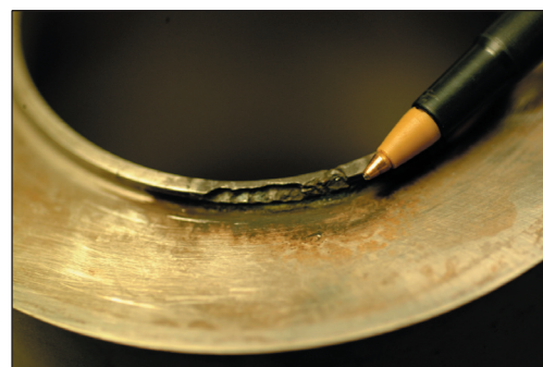
Exhibit 5-12. Arc damage to chrome plated parts.
