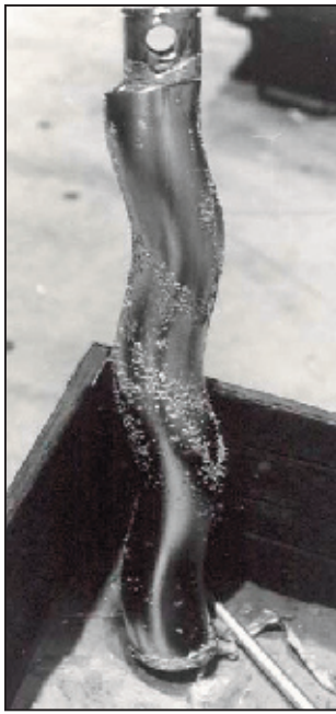
Exhibit 5-8. Peeled Chrome: A heavy buildup of chrome has blistered, indicating an adhesion problem.
